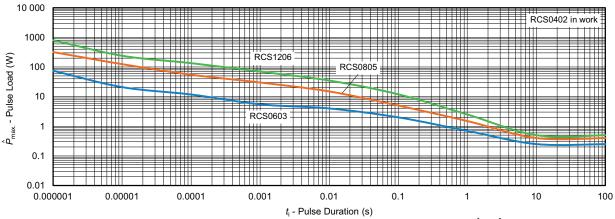
Maximum pulse load, continuous pulses; applicable if  $\overline{P} \leq P$  ( $\mathcal{G}_{amb}$ ) and  $\hat{U} = \hat{U}_{max}$ ; for permissible resistance change equivalent to 8000 h operation
