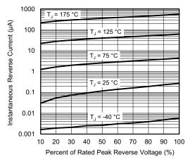
Fig. 4 - Typical Reverse Leakage Characteristics
