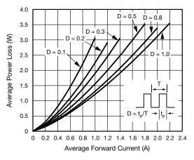
Fig. 2 - Average Power Loss Characteristics
