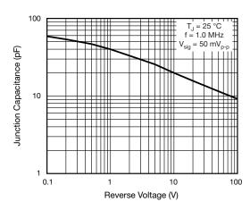
Fig. 5 - Typical Junction Capacitance
