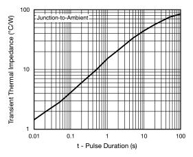
Fig. 6 - Typical Transient Thermal Impedance
