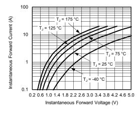
Fig. 3 - Typical Instantaneous Forward Characteristics
