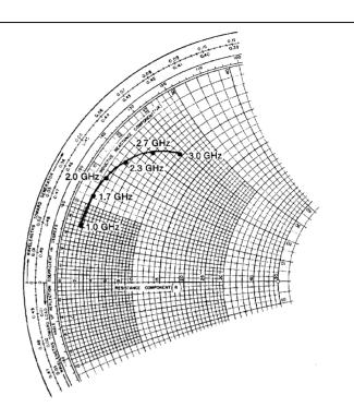
$P_{OUT} = Saturated$   $V_{CC} = 28V$ Normalized to 50 ohms
