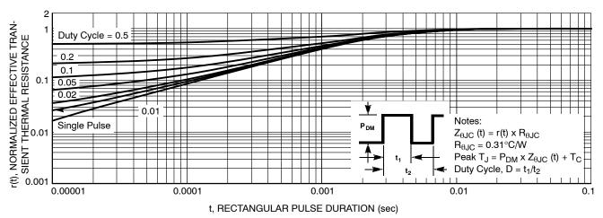
Figure 13. Junction-to-Ambient Transient Thermal Response Curve
