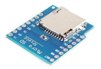
This shield is designed for use with the WeMos D1 mini and mini Pro development boards (see item HCWEMO0002). The shield provides a means of allowing a WeMos D1 mini to directly communicate with most types of microSD card. The shield is also compatible with the standard Arduino SD card library. The shield is supplied with 3 sets of headers (requires soldering) which allow for multiple...
