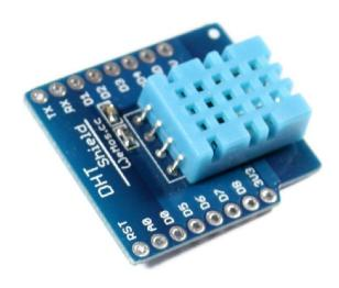
The DHT Shield is a digital temperature and humidity sensor shield based on the DHT11 sensor for your WeMos D1 mini. Measurements are read using one single pin. The measurement interval should be larger than 2 seconds.
