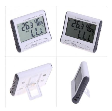
Brand : N/A Model : DC103 Quantity : 1 piece(s) per pack Color : White + grey Material ; Plastic Specification Temperature measuring range: indoor: -10'C~+50'C (+14'F~+122'F), outdoor: -50'C~+90'C (-58'F~+194'F); Humidity measuring range: indoor: 20%~99%; Power: 1 x LR44 (1.5V, not included); 2.9" LCD, with holder
