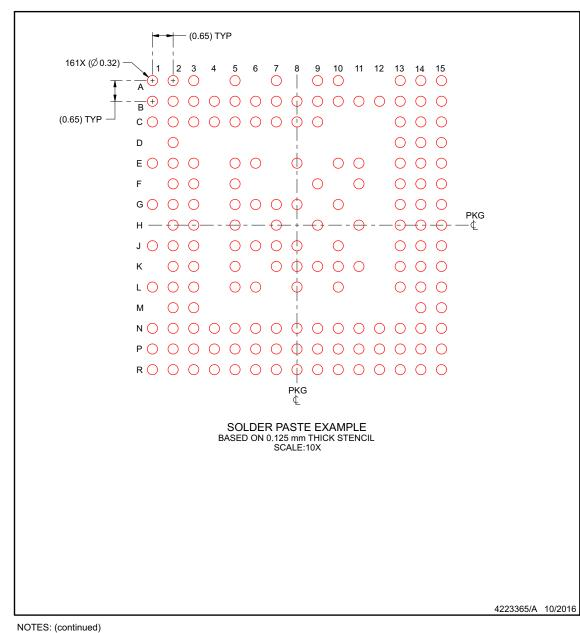
4. Laser cutting apertures with trapezoidal walls and rounded corners may offer better paste release.
