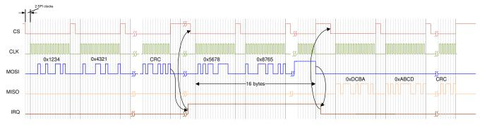
Figure 7-9. SPI Communication
