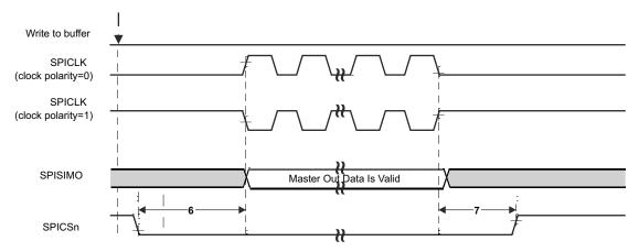
Figure 7-6. SPI Master Mode Chip Select Timing (CLOCK PHASE = 1)
