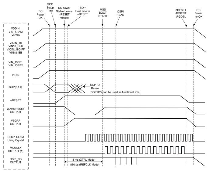
A. MCU\_CLK\_OUT in autonomous mode, where AWR6843 application is booted from the serial flash, MCU\_CLK\_OUT is not enabled by default by the device bootloader.
