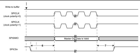
Figure 7-4. SPI Master Mode Chip Select Timing (CLOCK PHASE = 0)
