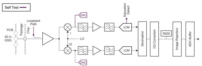
Figure 8-4. Receive Subsystem (Per Channel)
