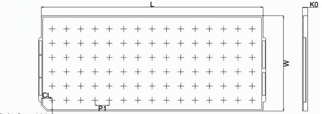
Chamfer on Tray corner indicates Pin 1 orientation of packed units
