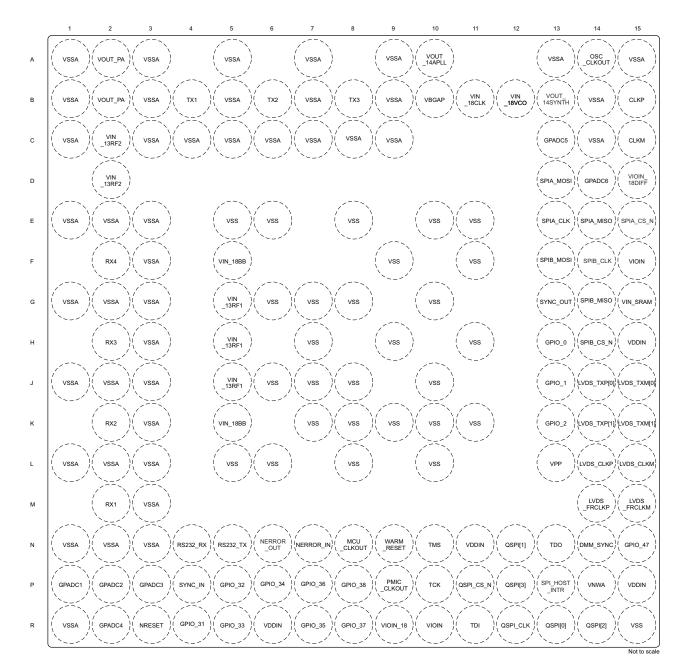
Figure 6-1. Pin Diagram
