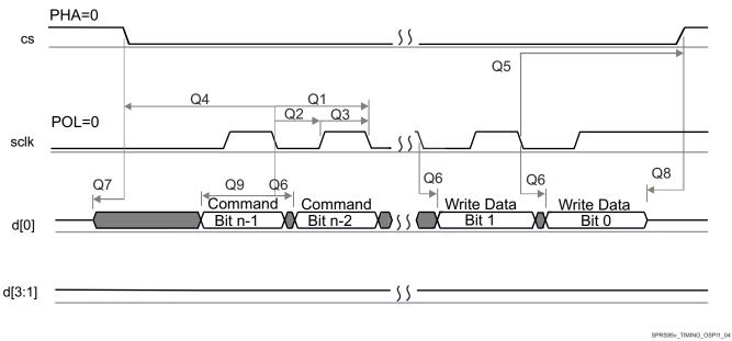
Figure 7-14. QSPI Write (Clock Mode 0)
