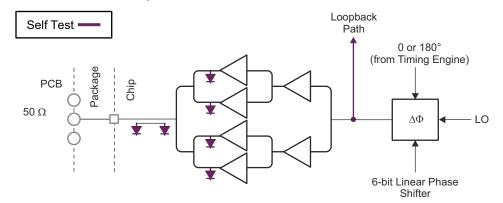
Figure 8-3. Transmit Subsystem (Per Channel)
