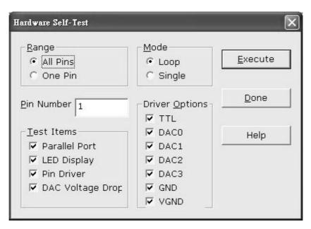
Manufacture recommend the user can run self-test of LABTOOL-48UXP prior to each day's operation. The self-test routine including testing the parallel port, LED display, Pin driver, TTL driver, relay, D/A converter's voltage drop and other parameter, following is the example test result screen.
