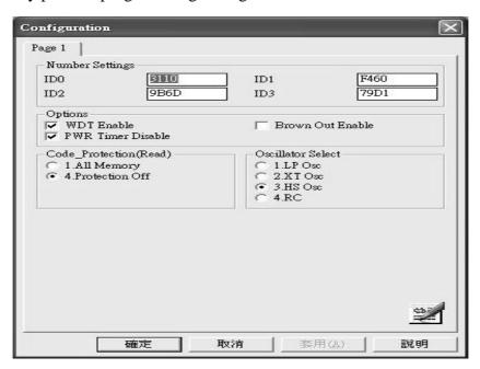
Figure 4-6 Example of device-specific configuration screen
