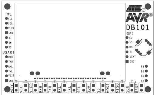
Figure 2-2. Assembly drawing of DB101 backside – backside view.
