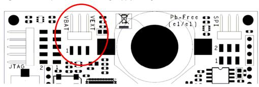
It is possible to sense whether the mega1281 runs from external supply or from battery as these voltages sources are connected to internal ADC of the mega1281. The ADC channels 0 to 4 (pins F0 to 4) are connected to various parts of the power supply network. Please refer to the schematics for more details on these connections.
