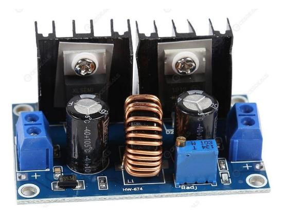
DC-DC Step-Down Power Supply Module XL4016E1 8A Adjustable Voltage Buck Regulator Board
