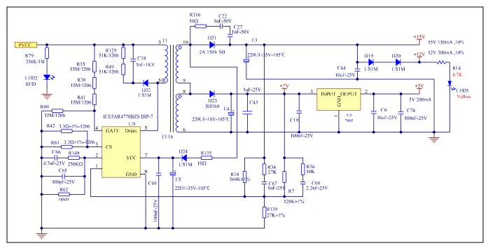
Figure 22 Power supply section of the REF-AIRCON-C302A-IM564 reference design
