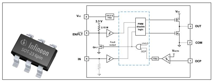
Figure 13 Package and block diagram of 1ED44175
