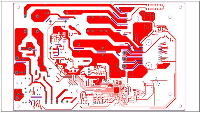
Top layer routing of the REF-AIRCON-C302A-IM564 Figure 24
