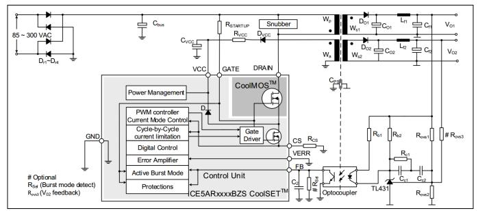
Figure 14 illustrates the internal block diagram and typical isolated flyback application.
