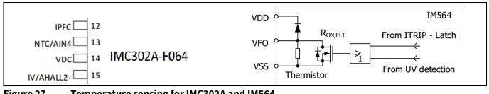
Figure 27 Temperature sensing for IMC302A and IM564
