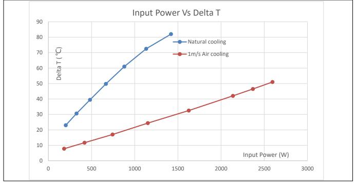
REF-AIRCON-C302A-IM564 thermal characterization (Input power vs IPM temperature Figure 26 rise)
