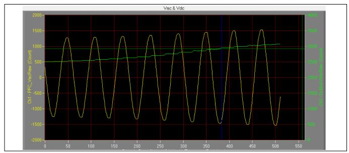
Figure 37 **OVP test by MCEDesigner trace function**
