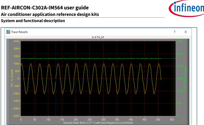
Figure 9 Trace waveform for Iu & Flx-M at 50% speed
