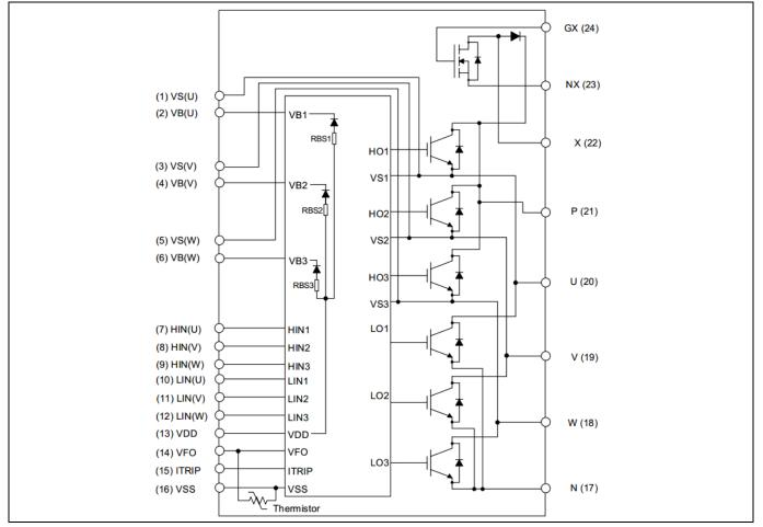
Figure 11 Block diagram of IM564-X6D
