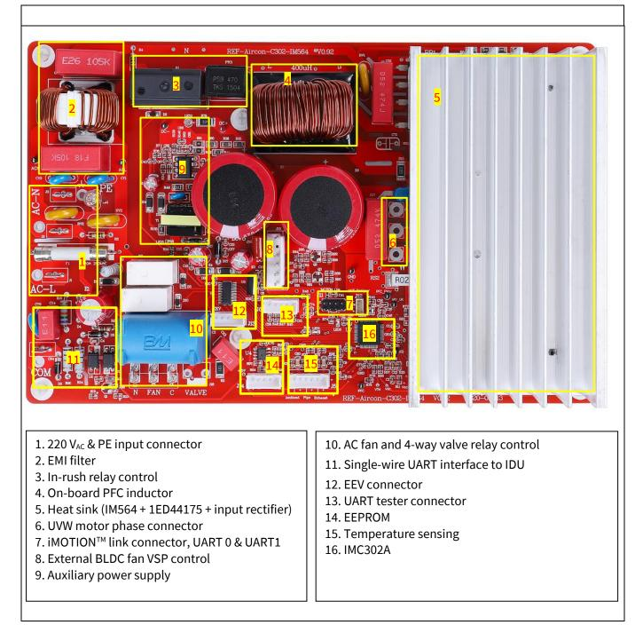
Figure 2 Functional groups of the REF-AIRCON-C302A-IM564 reference design
