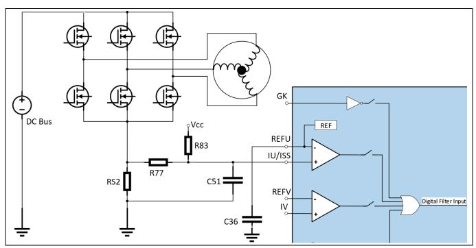
Figure 30 Overcurrent protection circuit on the REF-AIRCON-C302A-IM564 reference design
