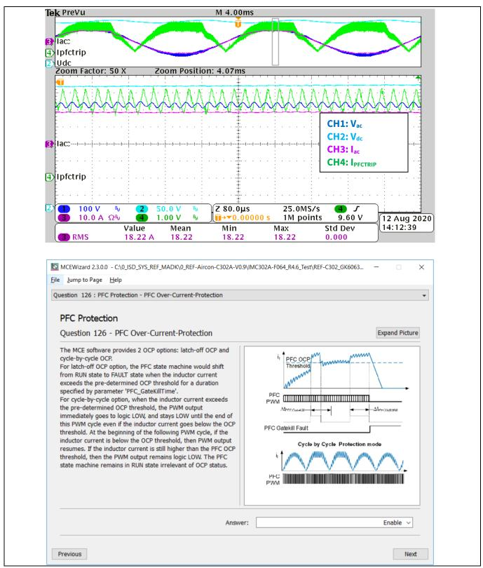
Figure 33 PFC Cycle-by cycle OCP test
