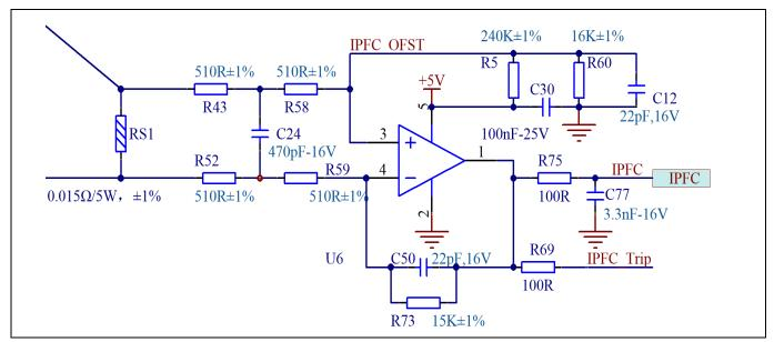
Figure 19 PFC current feedback with external op-amp
