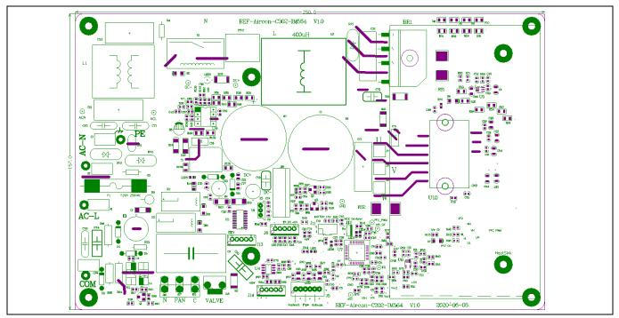
Figure 23 Top assembly print of the REF-AIRCON-C302A-IM564 reference design
