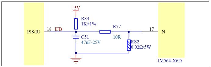
Figure 16 Direct AD sample (current feedback without external op-amp)
