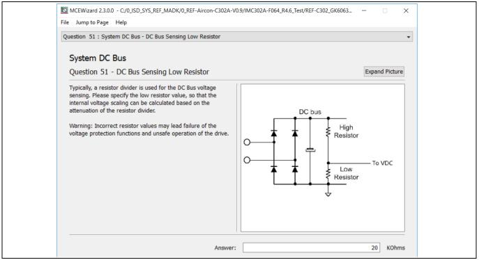
Figure 36 DC bus sensing configuration in MCEWizard
