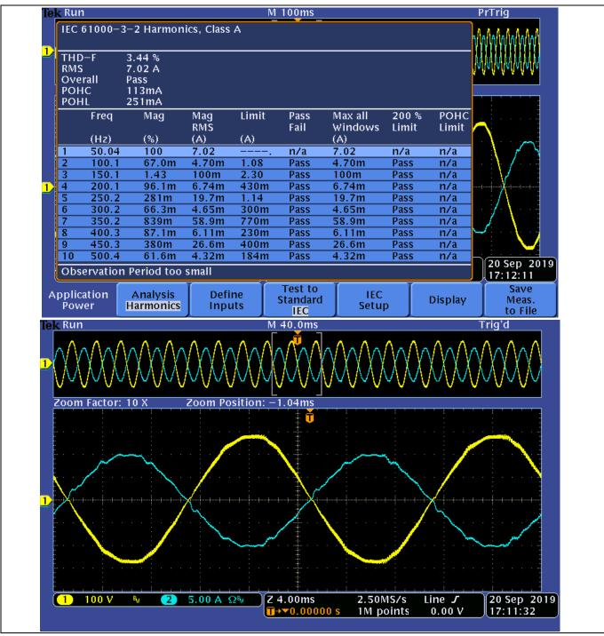
Figure 38 PFC performance test
