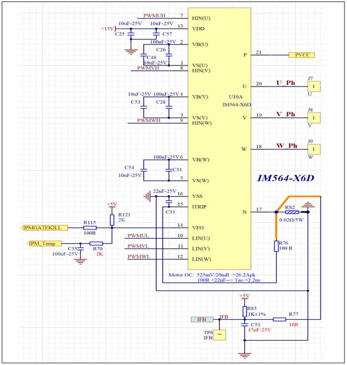
Figure 20 Inverter section of REF-AIRCON-C302A-IM564
