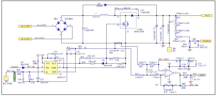
Figure 21 Schematics for PFC driver and current sensing
