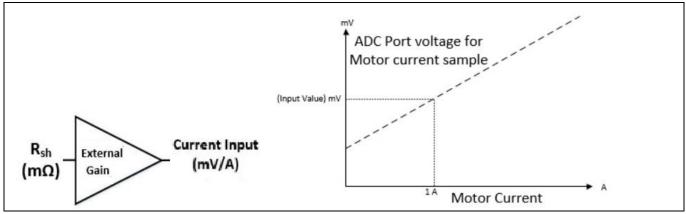
Figure 15 Current feedback scaling outside IMC302A
