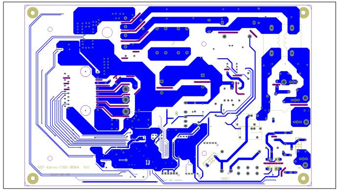
Figure 25 Bottom layer routing of the REF-AIRCON-C302A-IM564
