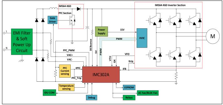
Figure 1 Block diagram of the REF-AIRCON-C302A-IM564
