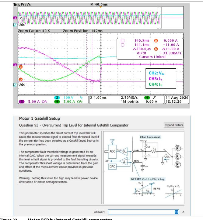
Figure 32 Motor OCP by internal Gatekill comparator
