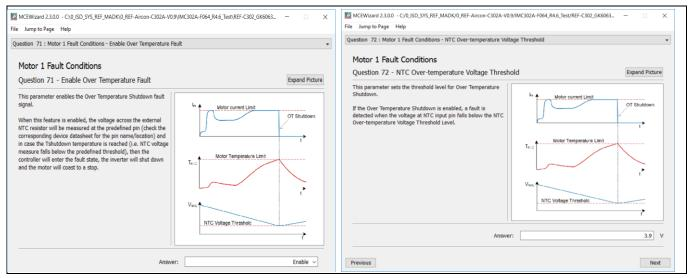
**Over-temperature protection enabled in MCEWizard** Figure 28
