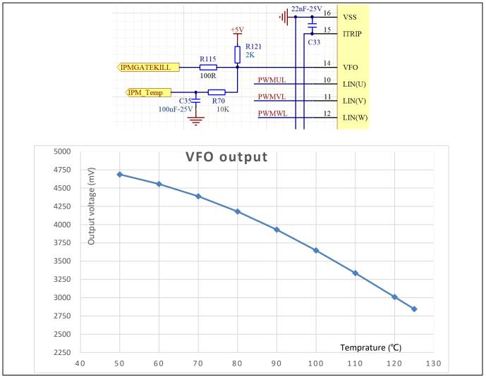
NTC circuit and output voltage curve Figure 29
