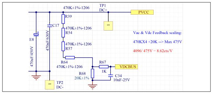
Figure 35 DC bus sense resistor on REF-AIRCON-C302A-IM564 reference design
