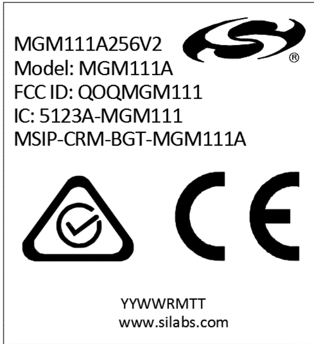
Figure 9.5. MGM111A Package Marking
