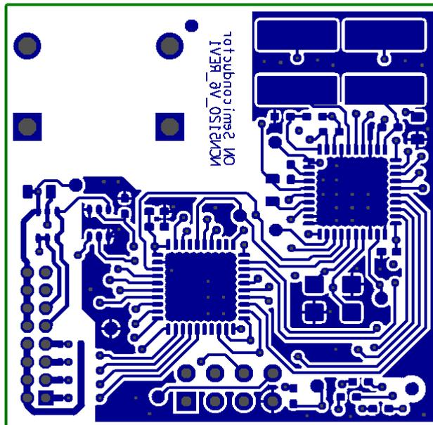
Figure 12. Bottom Layer of NCN5120 Reference Design
