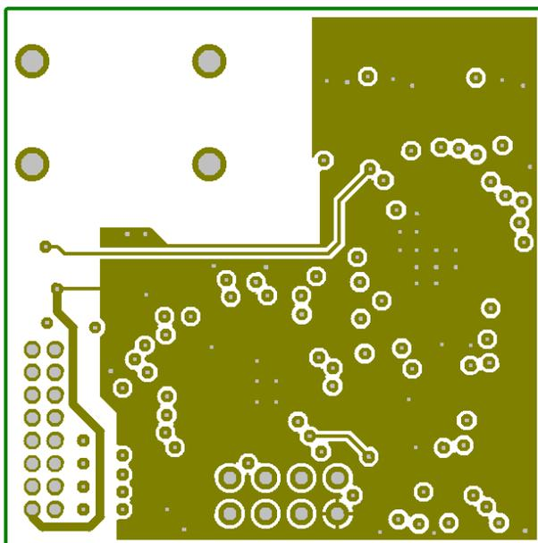
Figure 14. Inner Layer 2 of NCN5120 Reference Design
