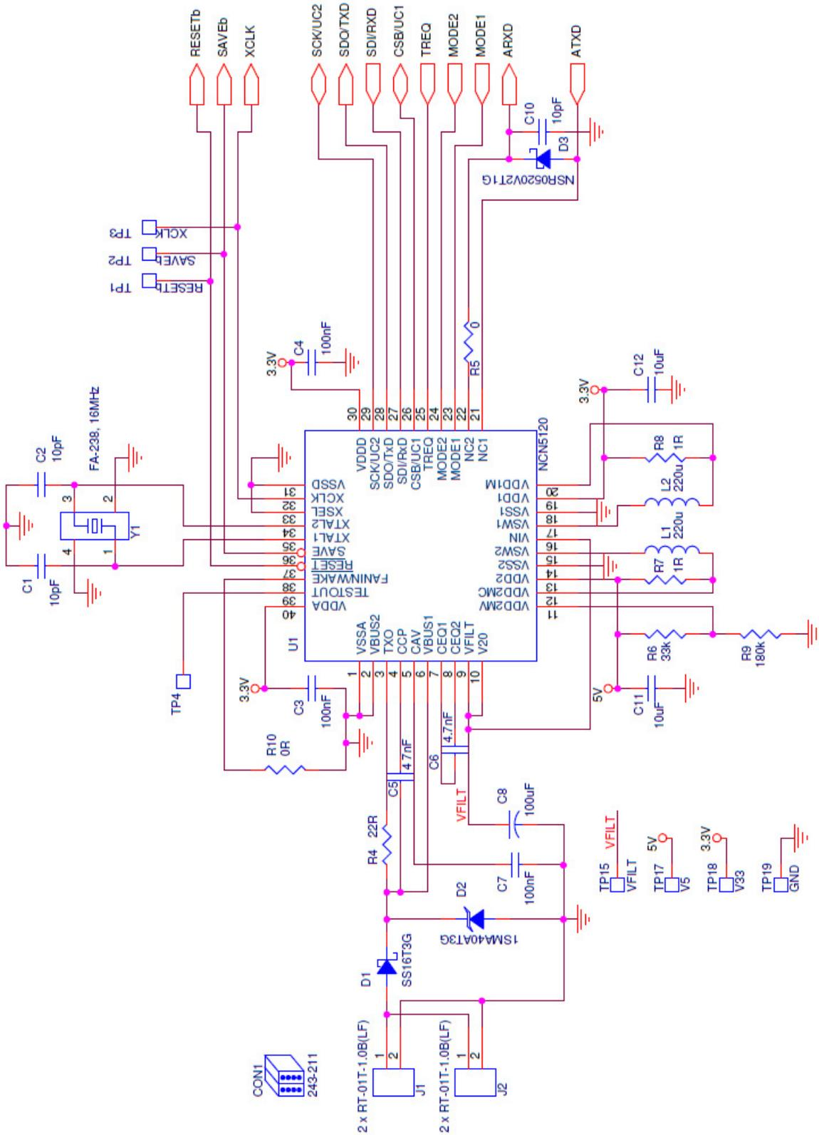
Figure 9. Schematic of NCN5120 Reference Design (Part 1)
