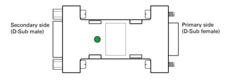
Figure 1: Top view PCAN-Optoadapter
