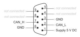
Figure 2: Pin assignment at the primary side (D-Sub female)
