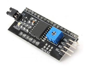
Interface Adapter Plate LCD1602 IIC/I2C is an LCD interface adapter for Arduino without the LCD screen. Since Arduino board I/O ports are limited usingInterface Adapter Plate LCD1602 IIC/I2C will let you add extra devices to your Arduino board. The module supports I2C protocol and the LCD contrast can be adjusted using the potentiometer on the board.
