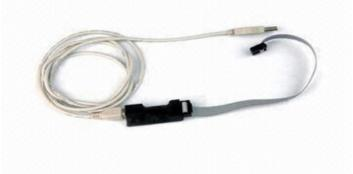
USB-powered Programmer TTPROG-B with Plug-and-play, 500mA Maximum Current and 150kbps Download Speed
