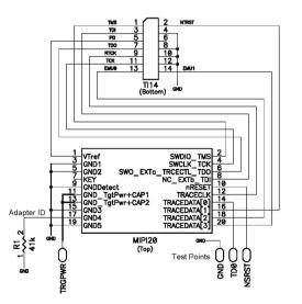
Figure 7: Diagram of the ADA-MIPI20-TI14 adapter
