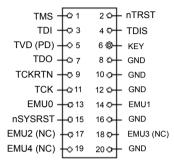
Figure 13: Pinout of the target cTI20 JTAG header
