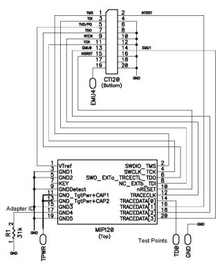
Figure 12: Diagram of the ADA-MIPI20-cTI20 adapter
