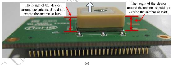
The device carry large amounts of interfering signals should be placed far away from the antenna, or should be shielded by shielding can.
