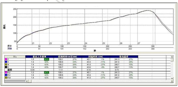
Figure 8: The Ramp-Soak-Spike reflow profile of SIM39EA
