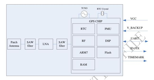
Figure 1: SIM39EA functional diagram
