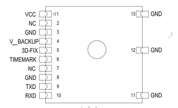
Figure 2: SIM39EA pin out diagram (Top view)
