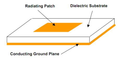
Figure 5: Basic features of GPS patch antenna
