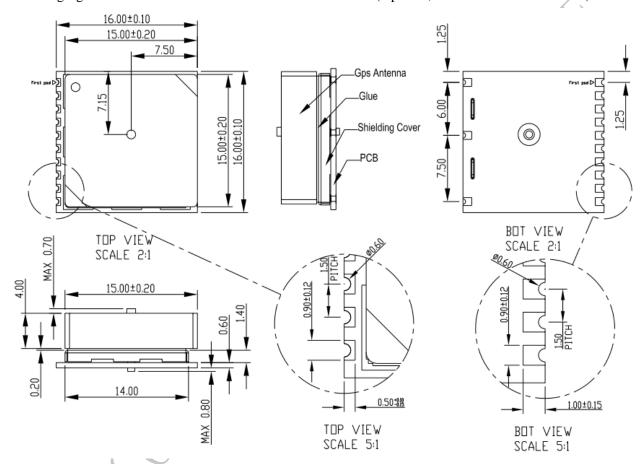
Figure 3: SIM39EA mechanical dimensions (Unit: mm)
