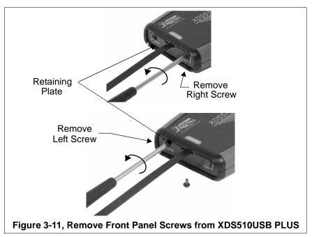
☐ Remove the cable retaining plate.
