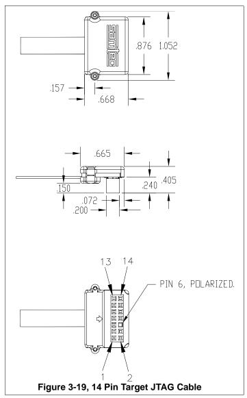
The target cable is flexible and about 13 inches long. It is made from micro coax cable. This type of cable has the following flex/bend limitations.
