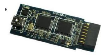
The XDS100v2 USB JTAG Emulator is the second release of the XDS100 JTAG emulator technology supporting debug of a variety of TI devices. The XDS100V JTAG connects to the PC via USB and to the microcontroller target board via the standard TI 14-pin (2x7) JTAG header. It is compatible with Code Composer Studio (CCS) V4 IDE from Texas Instruments and compatible with Windows 2000, XP, Vista (32-bit), and Win7 (32-bit).
