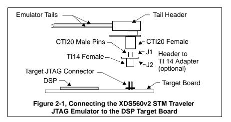
The figure below shows the factory installed configuration with the optional (CTI20 to TI14) adapter installed.
