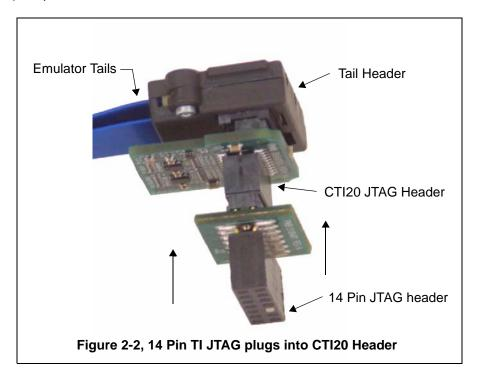
The adapter that comes with the XDS560v2 STM Traveler are shown in the figure below.
