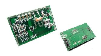
HW-M10 Microwave Motion Sensor PCB Module for Light Switch
