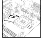
3. Lift the metal cover to expose the socket interior and place the socket in as shown.
