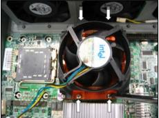
Remember to connect the power supply for the fan to complete the installation.
