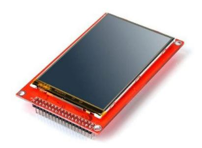
This TFT display is big (3.5" diagonal) bright and colorful! 480×320 pixels with individual RGB pixel control, this has way more resolution than a black and white 128×64 display, and double our 2.8" TFT.
