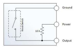
When a sufficient force is transferred to the switch, the terminal consisting of the spring moves and shorts both terminals together.
