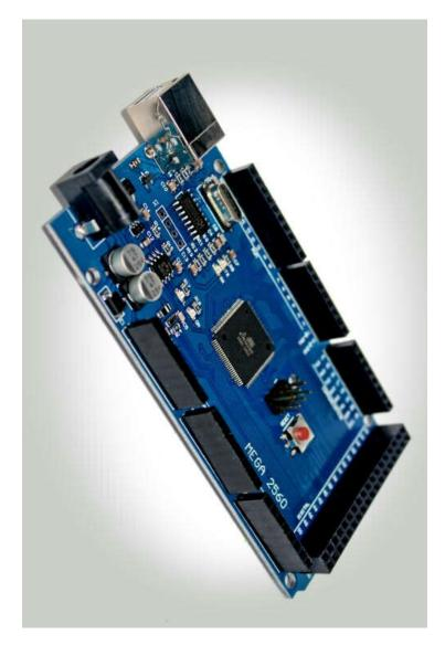
The Arduino Mega 2560 is a microcontroller board based on the ATmega2560. It has 54 Digital Input/Output Pins of which 15 can be used as PWM Outputs, 16 Analog Inputs, 4 UARTs Hardware Serial Ports, a 16 MHz Crystal Oscillator, a USB connection, a power jack, an ICSP header, and a reset button. It contains everything needed to support the microcontroller; simply connect it to a computer with a USB cable or power it with a AC-to-DC adapter or battery to get started.
