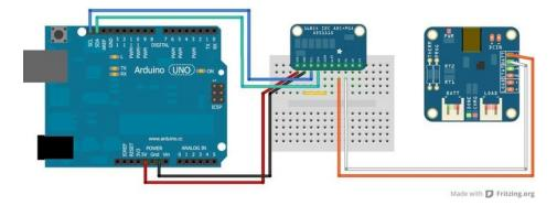
All input signals to these devices must be between ground potential and VCC. If your source signal produces negative voltages, they must be offset to fall within the GND to VCC range of the ASD1x15.
