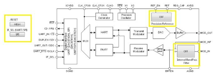
Figure 11. DAC8742HEVM Digital Input Selection
