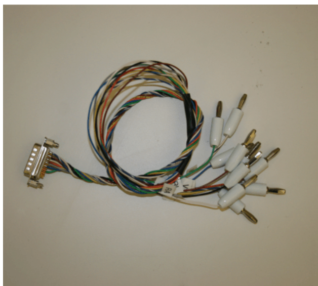
Figure 50. 15-Pin, Twisted Wire Cable to Banana Jacks
