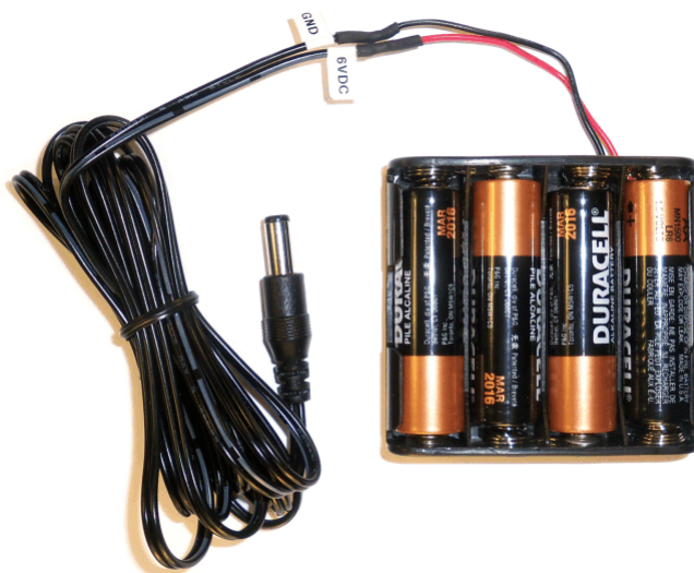
Figure 53. Recommended Power Supply for ADS1298R
