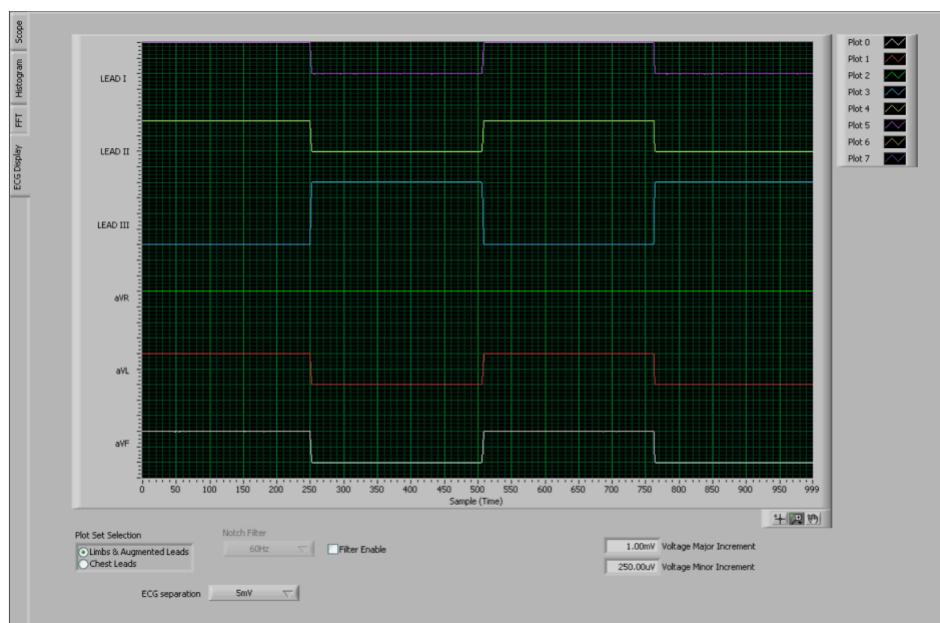
Figure 32. Example of Internal Test Signals Viewed on the ECG Display Tab
