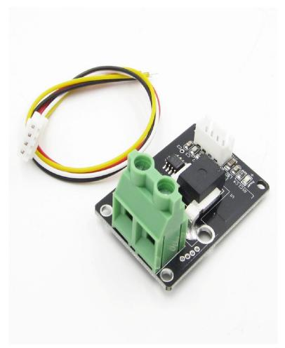
Bidirectional Current Sens module 120 kHz Bandwidth DC: -100-100A 0.02V/1A AC/DC ACS758LCB-100B Panel Mount +/-100Amp Current Sensor Board Detection Module
