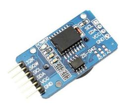
The DS3231 RTC High Precision Real-Time Clock Module is a low-cost, extremely accurate I2C real-time clock (RTC), it is more accurate than the ds1307 as this module is integrated with temperature-compensated crystal oscillator (TCXO) and crystal. The device incorporates a battery input, and maintains accurate timekeeping when main power to the device is interrupted.
