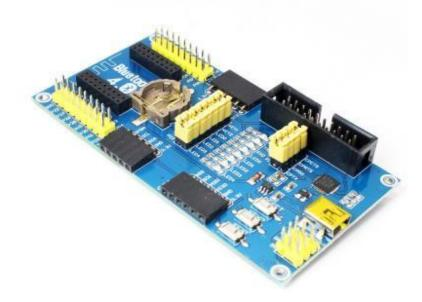
ble4.0 development board Bluetooth module nRF51822 backplane needs to be equipped with nRF51822 core board
