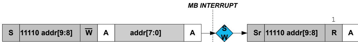
Figure 28-9. 10-bit Address Transmission for a Read Transaction
